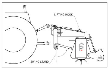
Figure 4. Swing Stand/Lifting Hook
